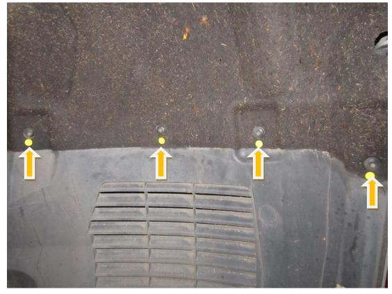
**6.** Again with your T25 torx drive remove the 7 fasteners that hold the lower arch spoiler in place to your undertray and arch liner.
