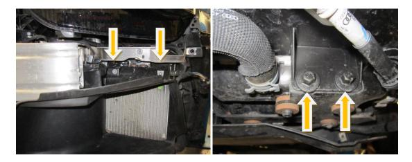
**13.** Using a T30 torx drive, loosen the fasteners that hold the headlight in place.
