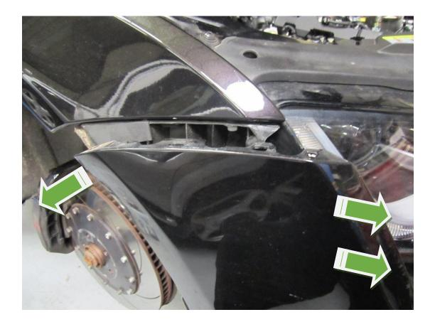
**9.** Using a T30 Torx drive remove the fastener that holds the bumper in place next to each front headlight .
