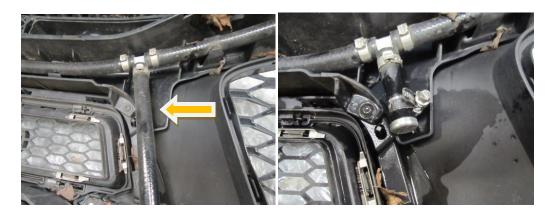
**29.** You must now tighten up the M8 allen caps that hold your new charge cooler radiator in place. Slide the radiator down towards the lower cowling leaving approx 1-3mm gap then fully tighten the radiator on the crash bar.
