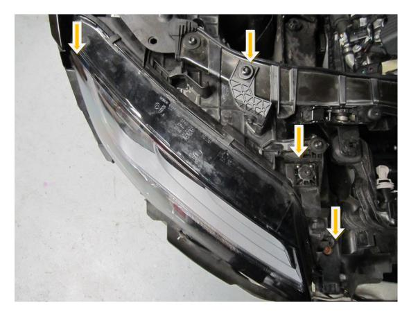
14. Disconnect the wiring loom from the back of your headlights then fully remove .
