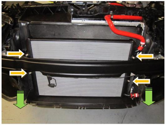
**30.** Part of your bumper must now be trimmed using a sharp knife or rotary grinder. Using a pen, mark the bumper then trim as per the photo below the area marked in red must also be cut out . Once trimmed, place the bumper in situ and hold in postion with the two torx fasteners you removed in section 9.
