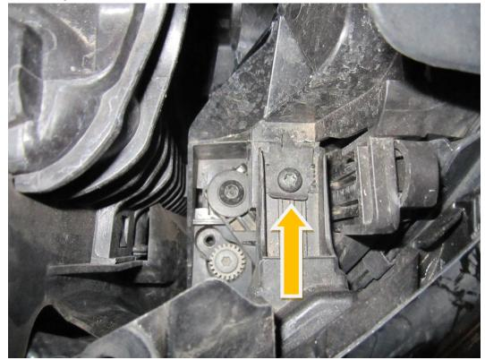
**10.** For the removal of the front bumper it is advised you have help so whilst one person pulls the bumper towards them they can then hold the bumper in situ while the other can disconnect various plugs on the wiring loom including the washer jets.
