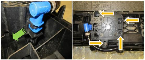
**28.** Taking care, with a sharp knife cut the washer jet pipe as pictured below then insert the 10mm blanking plug and secure in place with the hose clamp provided.
