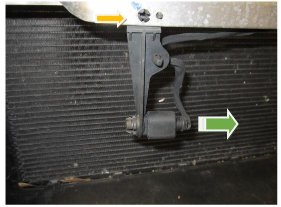
**16.** Using a 13mm spanner and socket remove the 13mm bolts either side of the crash bar that hold it in place, then fully remove.
