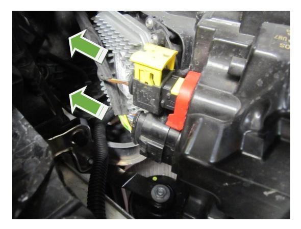
15. Remove the Air temp sensor from the crash bar and disconnect from the wiring loom .
