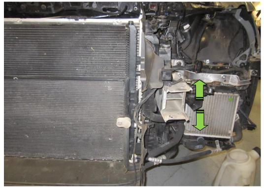
**20.** Remove the lower charge cooler hose arrowed in the picture below. You WILL lose the coolant within your OEM charge cooler radiator so a clean container is advisable to catch this in, then you can either re-use or dispose of correctly.
