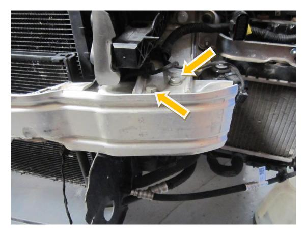
**17.** Remove the part of ducting arrowed and pictured below. This is to gain access to the lower charge cooler hose that must be removed .
