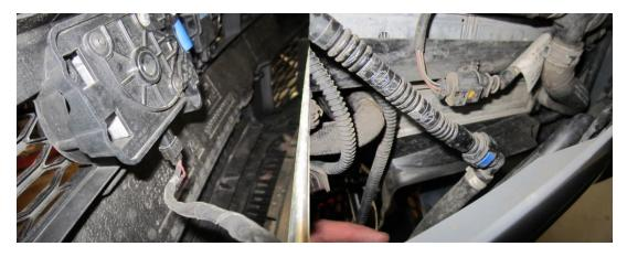
**11.** Remove the right hand part of the ducting (when viewed from the front of the vehicle) pictured below using a T30 torx Drive .This part is no longer required and can be discarded
