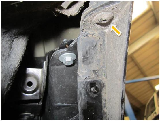
**8.** Pulling the arch away from the wing and towards the front of the car and unclip the sides of the bumper .
