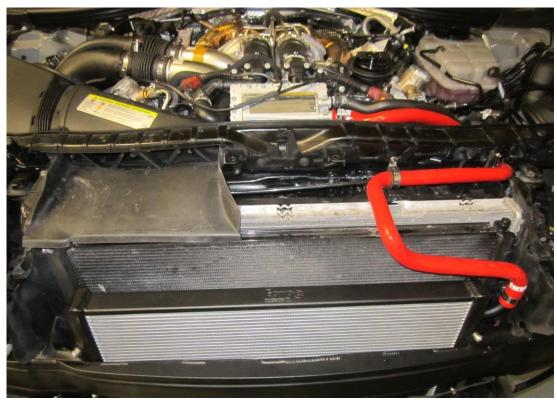
**26.** Fit the 25mm p-clip provided to hold the silicon hose in position.
