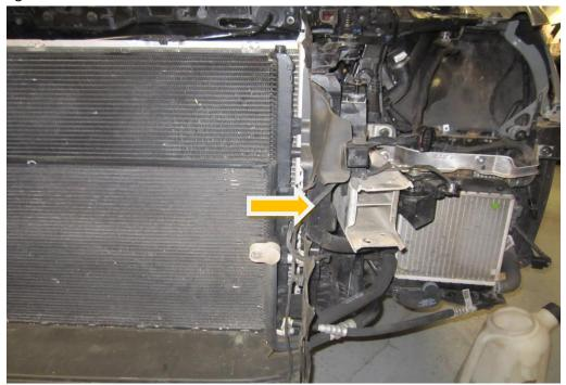
**18.** Fit your new Forge Motorsport radiator to the modified crash bar provided. Do not tighten the M8 allen cap bolts fully as there is adjustment that is needed in a few further steps.
