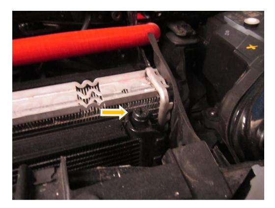
**32.** Keep checking your coolant level until fully bled .
