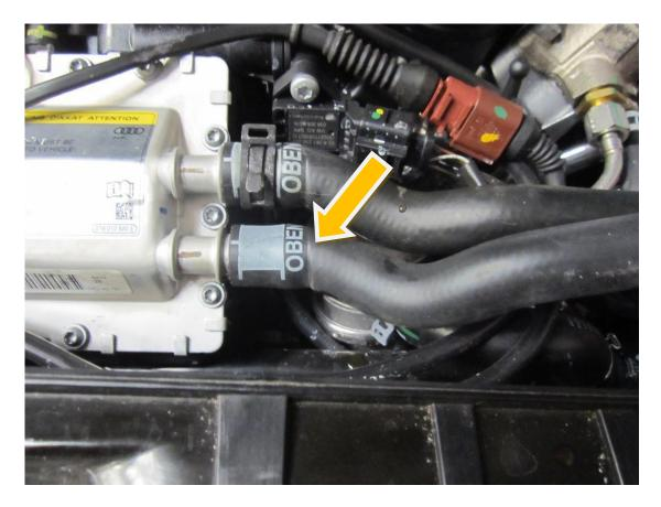
**25.** You can now fit the new upper Forge Motorsport silicon hose and tighten the hose clamps at both ends.
