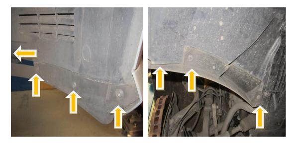
**7.** Using a T25 Torx driver, remove the fastener that joins the front corner of the bumper to the arch .
