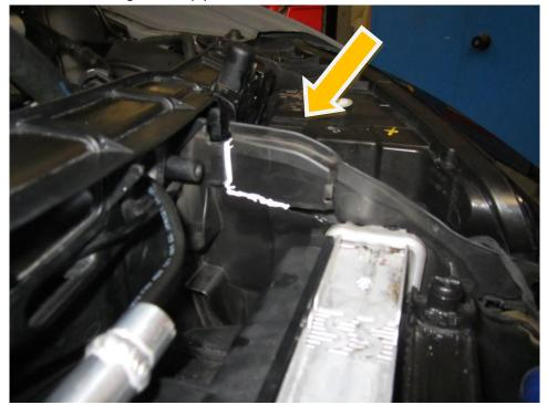
**22.** Where the lower Forge Motorsport charge cooler radiator lower pipe sits, a 40 mm hole must be drilled in the cowling as per the picture below .
