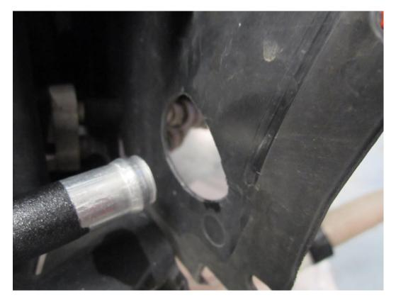
**23.** Fit the new Forge Motorsport silicon lower charge cooler hose into position and tighten the hose clamps both ends .
